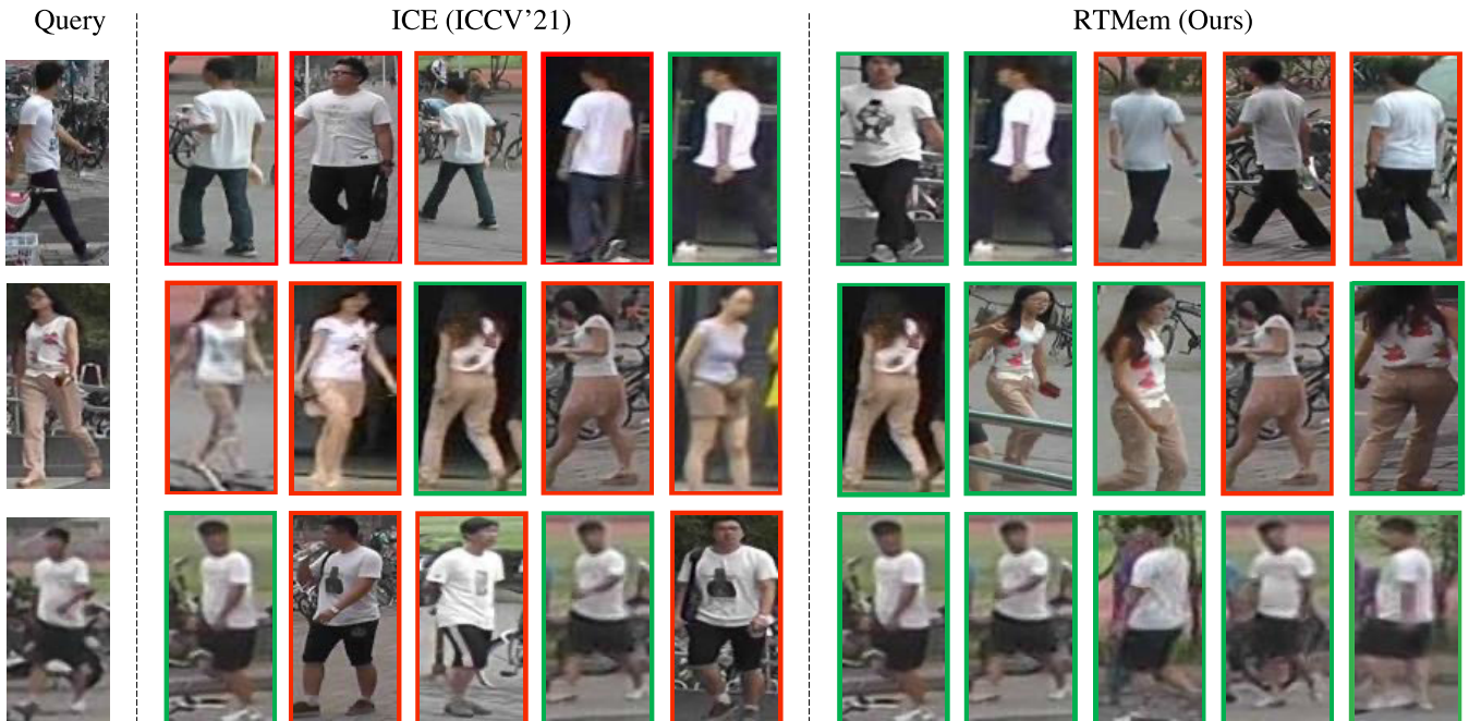
Fig. 8. Visualization comparison with ICE [19] and our RTMem on top five retrieved images on Market1501. Red boxes indicate false results, while green boxes represent correct results.
