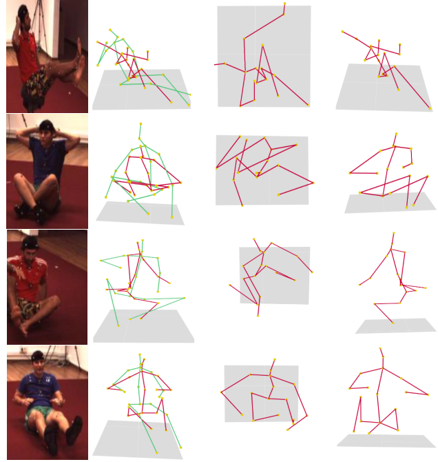
Figure 5. Failure cases on Human3.6M. 3D predictions with a P-MPJPE greater than 200mm. The first column shows the input images. The second column displays the predicted 3D pose (coloured in red) aligned with its respective ground truth (coloured in green). Following columns show different views of the predicted 3D pose.
