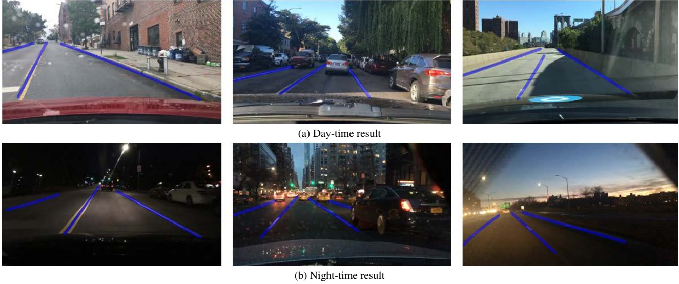
Figure 7. Visualization of the lane detection results of YOLOP. Top Row: Lane detection results in day-time scenes. Bottom row: Lane detection results in night scenes.
