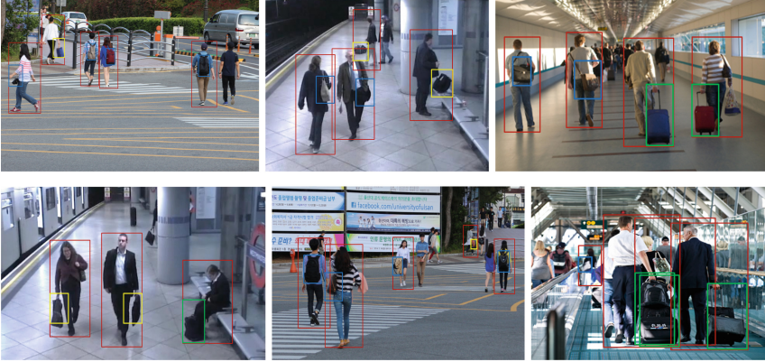
Fig. 4. Some typical detection results. The human-baggage object is detected as red bounding box. The baggage is then classified into category 1, 2 and 3 which are represented by blue, yellow and green bounding boxes, respectively (Color figure online).
