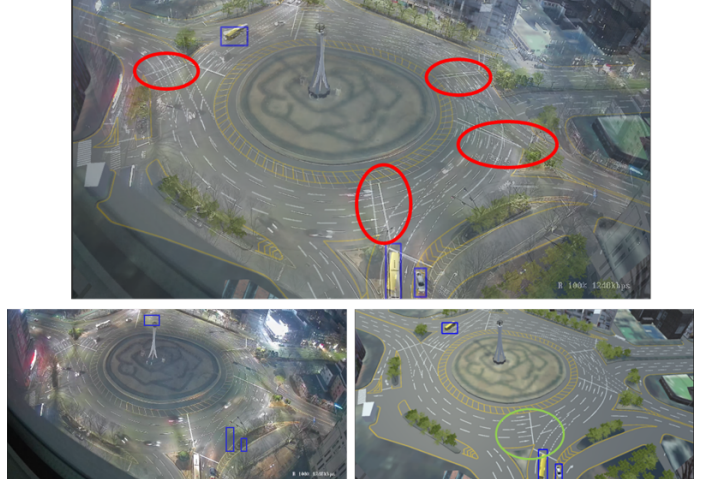
Fig. 1. Misalignment problem of images from digital twin and real. Blue bounding boxes on the left-bottom image from real environment are generated by YOLOv8 [1] trained with VisDrone [2] dataset. Bounding boxes on the right-bottom image from virtual environment are generated by just mapping those from real image to twin image. The image above is made by overlap two bottom images. Red ellipses show the misalignment between the images captured on real camera and digital twin camera. Because of this problem, the vehicles in the green circle are placed in the wrong position, compared with vehicles in left-bottom image.
