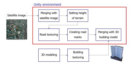
Fig. 1. Digital twin building process.
