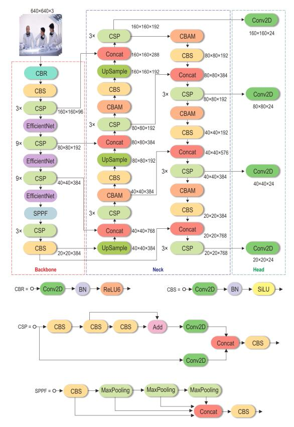
Fig. 1. The proposed network architecture overview and sub-modules.
