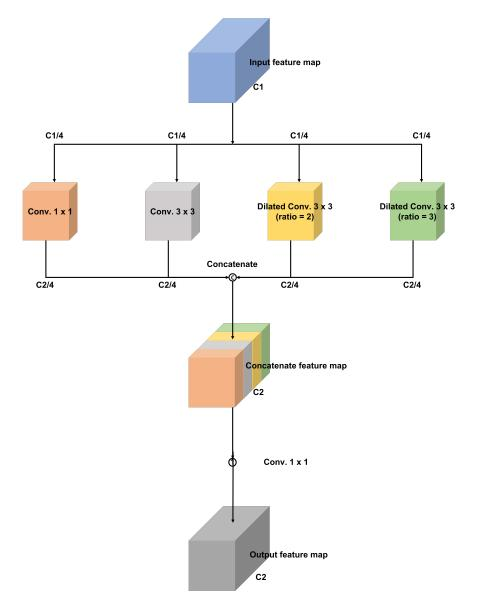
Fig. 4: Illustration of the proposed Dilated Depth-wise module.
