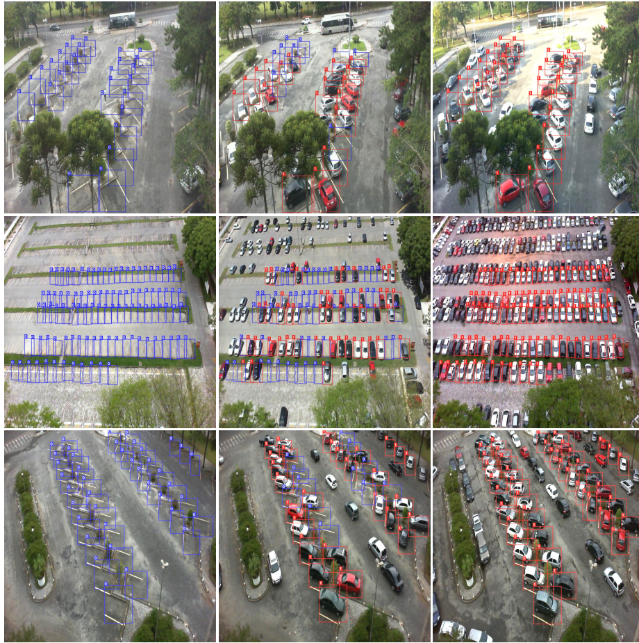
Fig. 6. The qualitative results of the proposed network on the test set of PKLot dataset with IoU threshold = 0.5. The numbers denote the classes: 0 is space-empty, and 1 is space-occupied.
