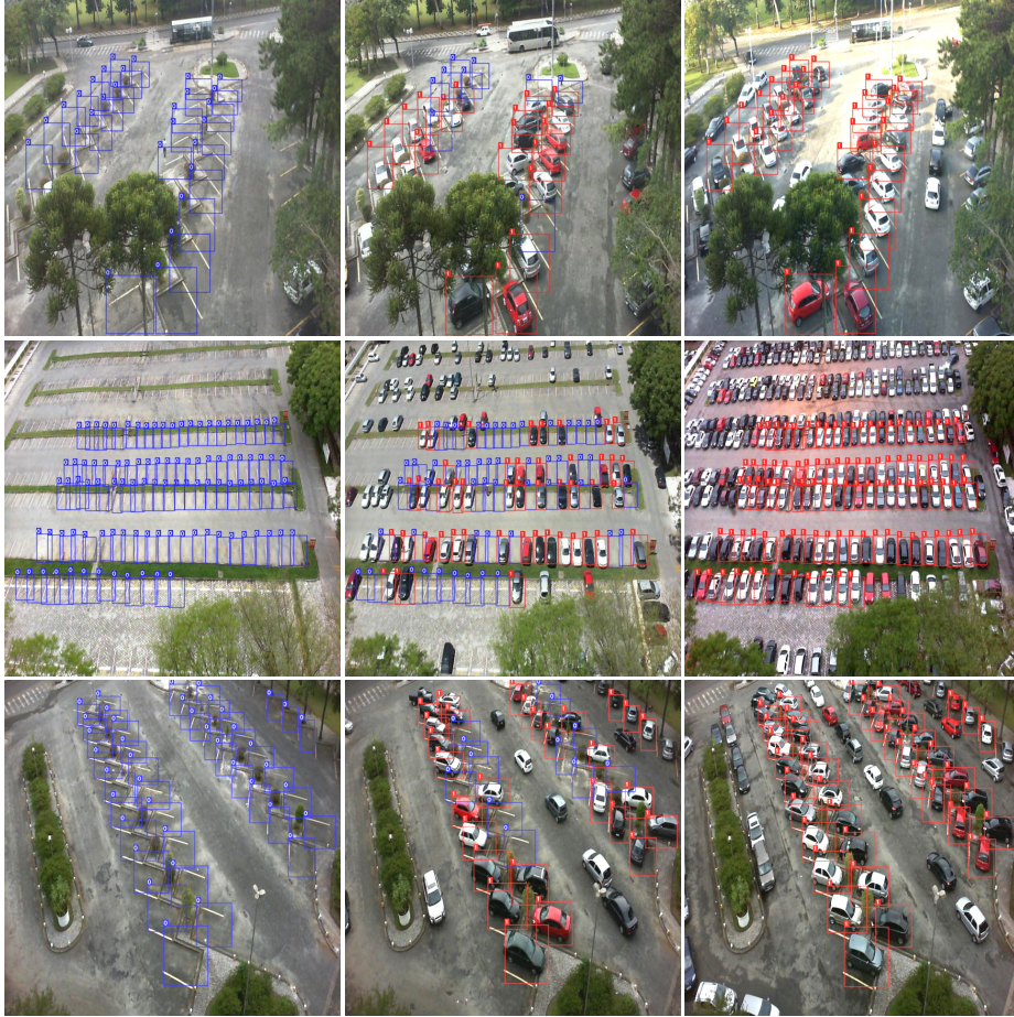
Fig. 6. The qualitative results of proposed network on the test set of PKLot dataset with IoU threshold = 0.5. The numbers denote the classes: 0 is space-empty, 1 is space-occupied.
