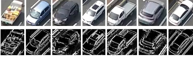
Fig. 4: Generated edge image for cropped vehicle area; first row: cropped image in the original, second row: edge image from a cropped image.
