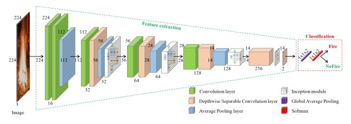
Fig. 1. The proposed fire classification network. This network consists of two sub-modules: feature extraction and classification.
