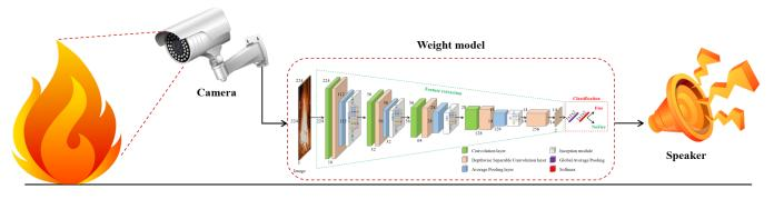
Fig. 3. The overall of fire video testing system. This system consists of camera, trained weight model, and speaker.
