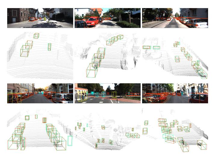
Figure 3: Qualitative results of the proposed method using the KITTI validation dataset. In the RGB images, the red, cyan, and yellow color represent the predictions for the car, pedestrian, cyclist, respectively. In the point cloud images, the green color denotes the ground truth, and the red color represents the prediction. The results in the point cloud images are used for a qualitative comparison.
