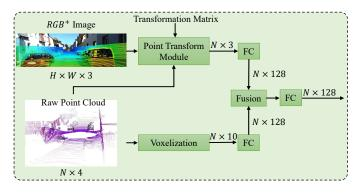
Figure 2: Visualization of the point feature fusion module. N is the number of points in a point cloud, and FC denotes one fully connected layer.
