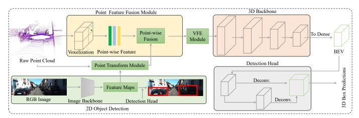
Figure 1: The architecture of the proposed one-stage 3D object detection network for the LiDAR and camera. It mainly includes the input data, the point feature fusion module, the 3D backbone, the 2-D object detection and the detection head. The gray box and green box represent the convolutional block and feature map, respectively.
