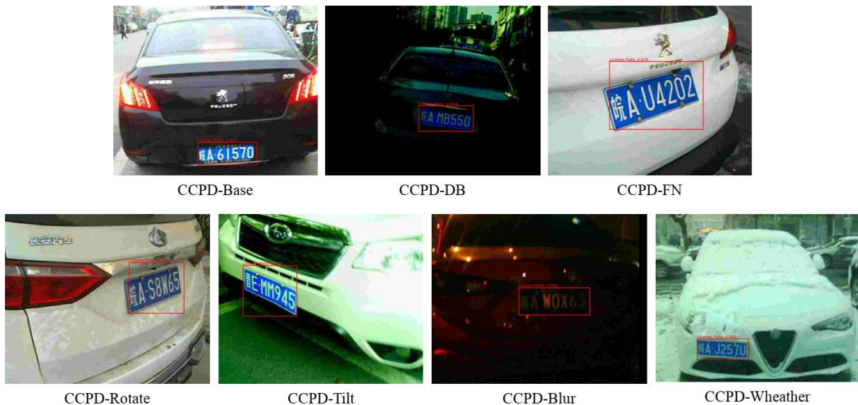
Fig. 3. The qualitative result of license plate detection network on CCPD dataset.
