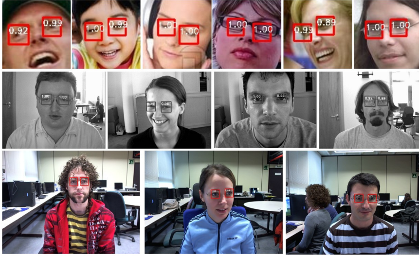
Fig. 5. The qualitative result on CEW dataset (first row), on BioID Face dataset (second row), and on GI4E dataset (third row). The proposed network can detect eye location at many different pose shown as in CEW dataset and when wearing the glasses shown as in BioID Face and GI4E dataset. The number in each bounding box shows a confidence score of prediction.
