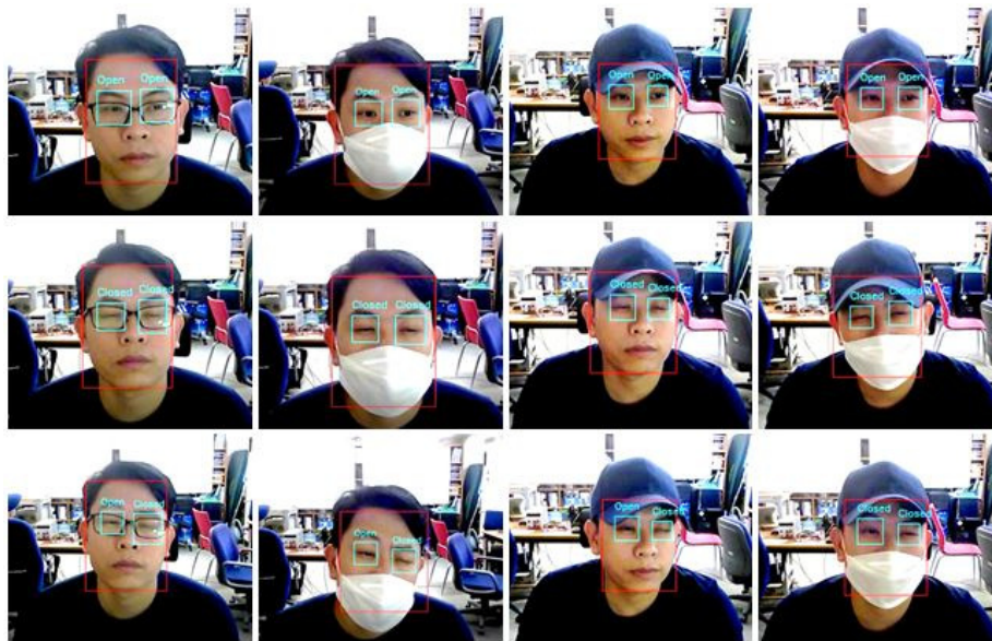
Fig. 7. The qualitative result when testing on camera connects with Jetson Nano device with four situations: glasses (first column), face mask (second column), hat (third column), face mask and hat-wearing (fourth column).
