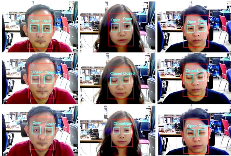
Fig. 6. The qualitative result when testing on camera connects with Jetson Nano device with three participants (two males and one female). The result shows in two open eyes (first row), two closed eyes (second row), one closed eye and one open eye (third row).
