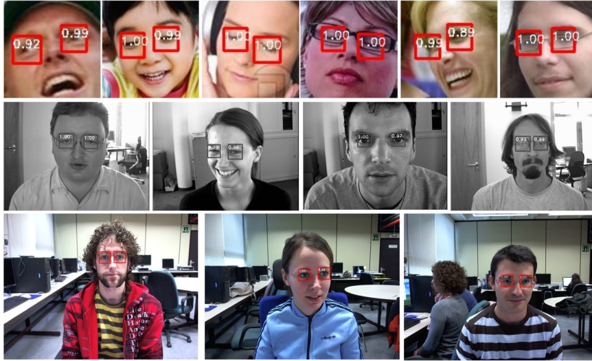
Fig. 5. The qualitative result of the eye detection network on CEW dataset (first row), on BioID Face dataset (second row), and on G4E dataset (third row). This network can detect eye location in different situations: head poses, the glasses-wearing, laboratory environment. The number in each bounding box shows a confidence score of prediction.
