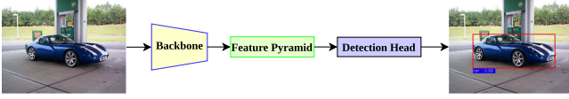
Fig. 2. Overall architecture of the BBENet consists of three parts: backbone network, feature pyramid, and detection head. The backbone network extracts the informative features from the input image. The feature pyramid constructs multilevel feature maps with different scales. The detection head predicts classification scores and bounding boxes for each object in the image.
