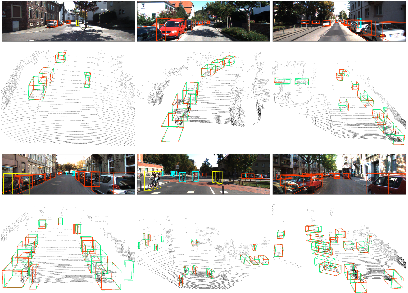
Figure 6: Qualitative results of the proposed method using the KITTI validation dataset. In the RGB images, the red, cyan, and yellow color represent the predictions for the car, pedestrian, cyclist, respectively. In the point cloud images, the green color denotes the ground truth, and the red color represents the prediction. The results in the point cloud images are used for a qualitative comparison.
