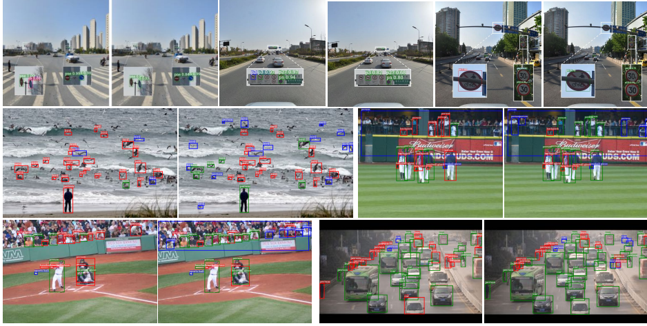
Fig. 5. Qualitative examples comparison between base model FPN and our EFPN on Tsinghua-Tencent 100K (row1) and MS COCO (row2&row3). The right in each pair denotes FPN results, while the left denotes EFPN results. The red boxes represent false negatives, the blue boxes represent false positives, and the green boxes represent true positives. Detectors of traffic-signs and general objects both profit from EFPN on challenging small object detection
