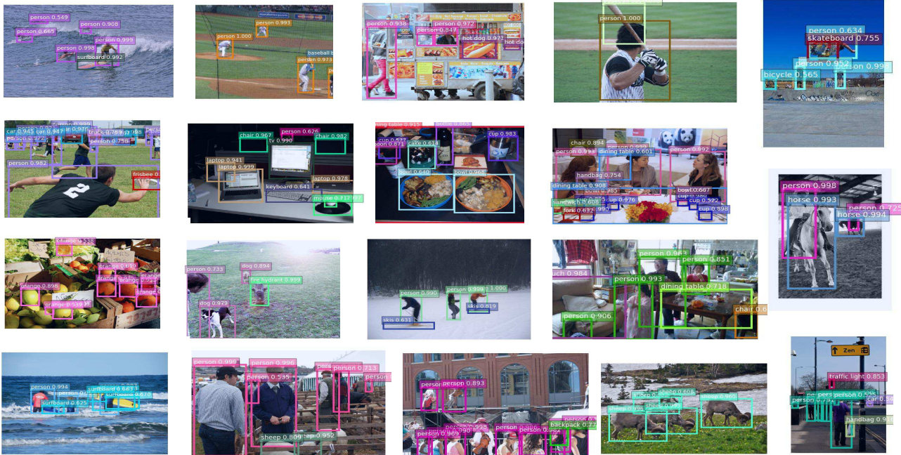
Figure 4. Example of object detection results on the MS COCO test-dev set. The training data is COCO trainval. Each output box is associated with a category label and a softmax score in [0, 1] . A score threshold of 0.4 is used for displaying.
