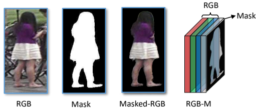
Figure 4. Different inputs for person ReID. With the binary mask, we can generate a synthetic RGB+Mask pair (RGB-M in short), including three RGB channels and one mask channel.
