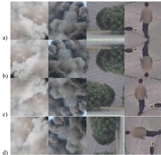
FIGURE 2. An example of data augmentation. a) Original images in the training set; b) Corresponding new images generated by horizontal flip; c) Corresponding images by vertical flip; d) Corresponding images rotated by 90 degrees.
