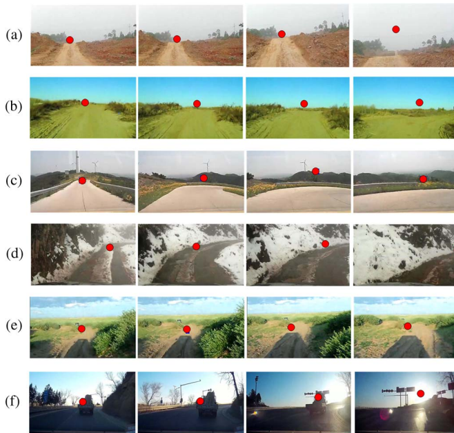
Fig. 9. Illustrations of how the vanishing point fails under poor road conditions (a), no-road situations (b)–(d), or when there are strong shadows or sun glare in the road images (e), (f).
