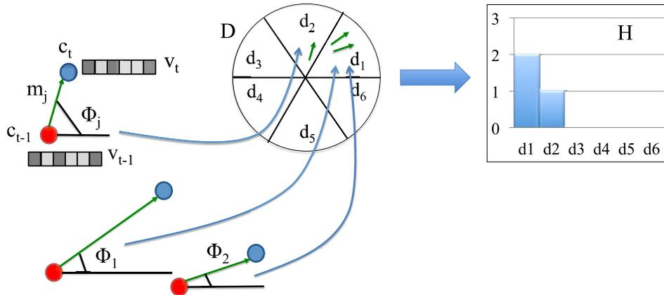
Fig. 4. Given the corner points  $c_{t-1}$  and  $c_t$  (red and blue circles, respectively), the matching  $m_j$  is obtained by minimizing the Euclidean distance between the corresponding descriptors  $v_{t-1}$  and  $v_t$ . The direction of the motion, encoded by the angle  $\phi_j$ , is evaluated according the dictionary  $D$ , and the histogram of occurrences  $H$  is then built.
