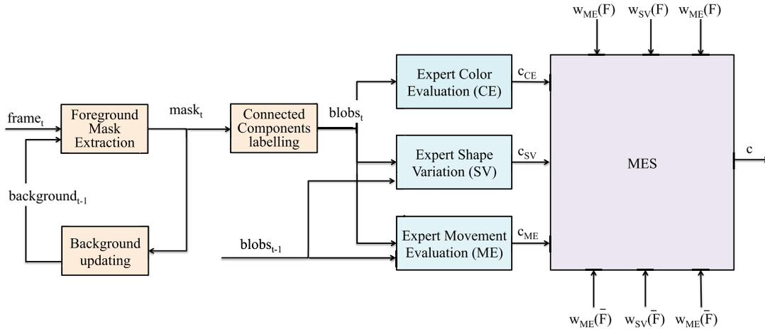
Fig. 1. Overview of the proposed approach. The blobs are detected by a background subtraction algorithm; the decision is taken by combining the information coming from three different experts, which are respectively, based on color, shape variation, and motion that analyze every input blob. Note that the last two experts need to be supplied with the blobs detected at the current frame and the previous frame.
