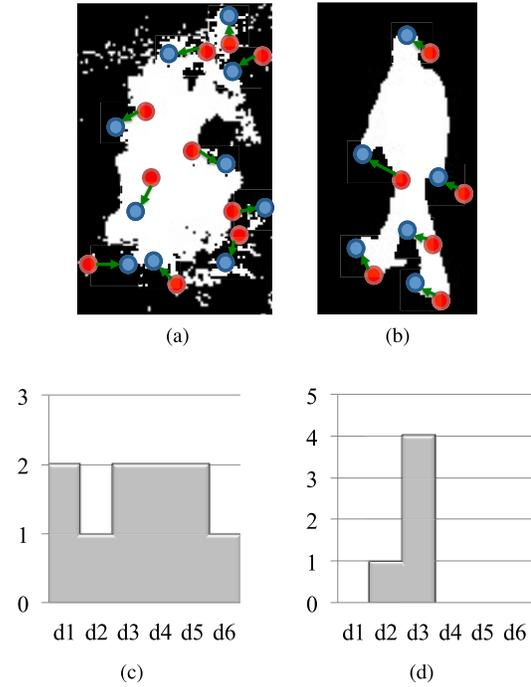
Fig. 3. Low level representation (a), (b) and high level representation (c), (d) of a fire (a), (c) and a non fire (b), (d) blob. Red and blue circles in (a) and (b) represent the salient points extracted at the frame  $t$  and  $t - 1$ , respectively.
