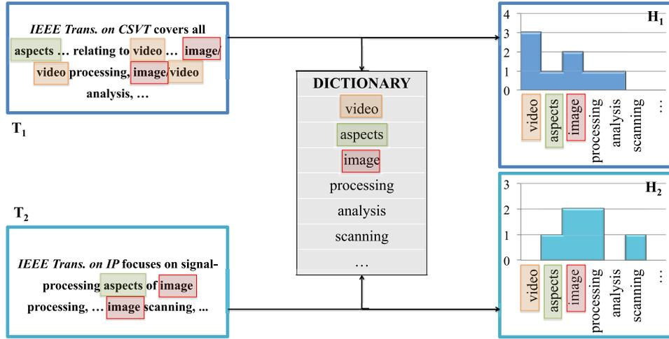
Fig. 2. Rationale of the bag-of-words approach applied to text classification: the occurrences, in a document, of a predefined set of words included into a dictionary are used for building up a histogram of occurrences. See the histograms  $H_1$  and  $H_2$  associated with the texts  $T_1$  and  $T_2$ , respectively.
