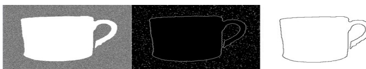
Fig. 4. Left: Noisy input image Middle: Output of Sobel edge detector Right: Output of our algorithm.
