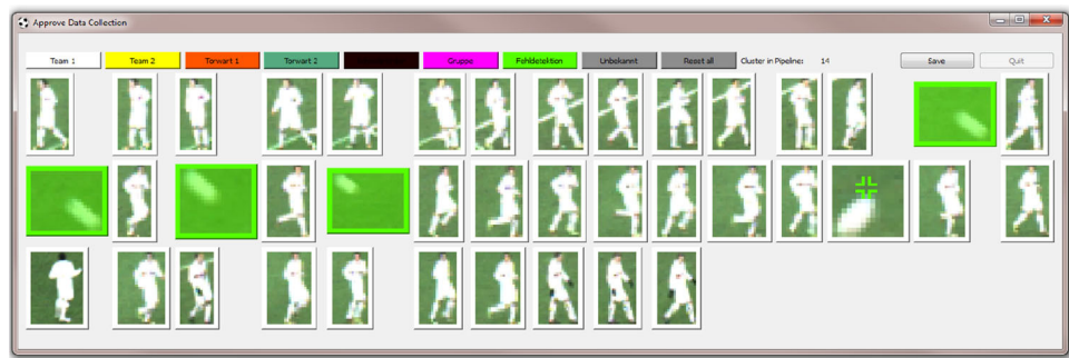
Fig. 14 Operator interface for the assignment of pre-sorted object clusters to the trained classes. The shown cluster is assigned to one of the classes indicated by the colored buttons in the top row . Examples that do not fit this class are labeled individually. By confirming the dialog, the assignments are sent to the processing machine
