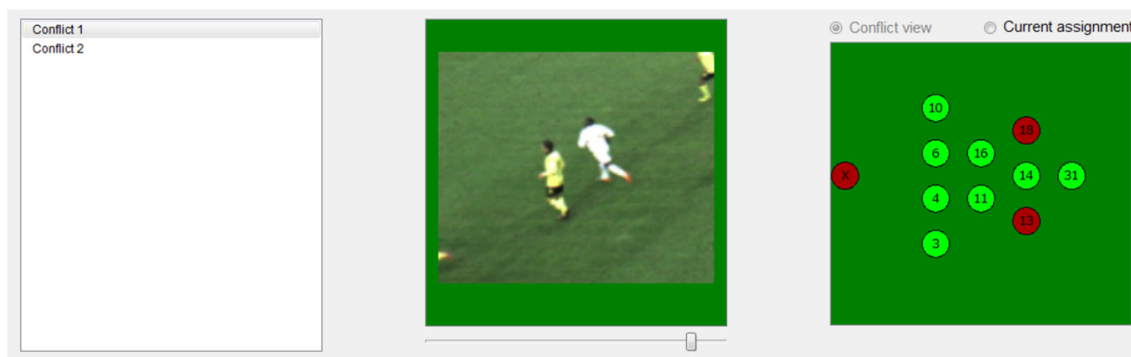
Fig. 16 Conflict review: the operator is presented a video clip of the missed situation and corresponding team assignments—again one click solves the problem
