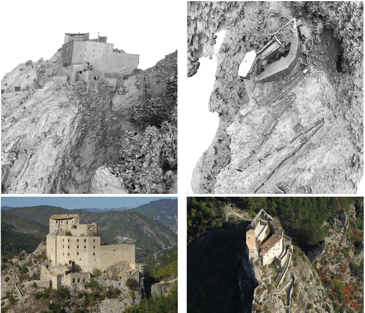
Fig. 12. Results on Entrevaux data set. Nontexture mesh from 109 images taken from a helicopter (© IMAGINE/CSTB), seen in two views associated with similar images.
