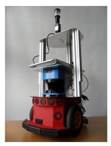
Fig. 1: Pioneer 3-DX equipped with an omnidirectional camera
