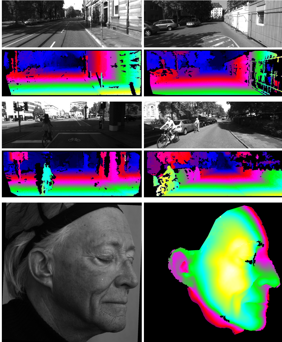
Fig. 6. Challenging urban scene and face dataset. We evaluate our algorithm on an urban video sequence at 1382 \times 512 pixels resolution. By computing disparity maps at 2 fps and using visual odometry with sparse features, we were also able to obtain a 3D scene reconstruction in real time (see http://www.cvlibs.net ). The bottom row shows a one Megapixel face image from the dataset of [26] and the corresponding disparity map obtained using our algorithm. Best viewed in color.
