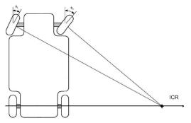
Figure 2. General Ackermann steering principle
