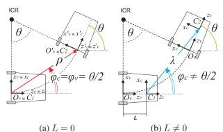
Figure 3. Camera and vehicle motion under circular motion constraint. When camera and vehicle reference systems coincide  $\varphi_c = \varphi_v = \theta/2$  (a). When the camera has an offset L with the vehicle's origin, we still have  $\varphi_v = \theta/2$  but  $\varphi_c \neq \theta/2$  (b). Note, the camera does not necessarily have to be on the axis of symmetry of the vehicle.
