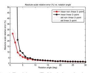
Figure 4. The relative error % of the absolute scale estimate as a function of the rotation angle  $\theta$ . Comparison between the linear 3-point method (circles) and the non-linear 2-point method (squares).
