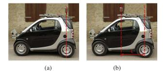
Figure 1. If the camera is located on the vehicle's non steering axle, the rotation and translation of both the camera and the car are exactly the same (a). If the camera is mounted with an offset to the axle, rotation and translation of camera and car are different (b). While case (a) can be used to simplify motion estimation (see our previous work [12]), case (b) can be used to compute the absolute scale from a single camera.
