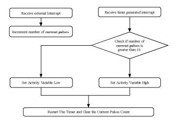
Figure 4. Algorithm for load detection
