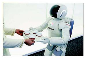
Figure 12. ASIMO Service robot from Honda
