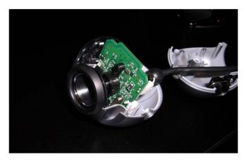
Figure 15. The camera and associated circuit of the robot for vision
