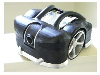
Figure 13. Fabricated robot for home monitoring
