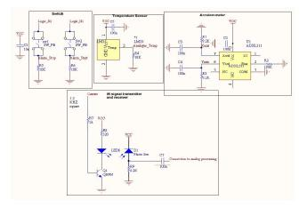
Figure 9. The electronic circuit of the sensor unit
