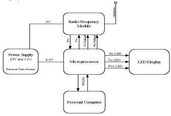
Figure 5. Core components of the Central Controller Unit (CCU)
