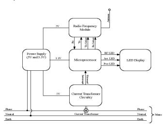
Figure 3. Core components of the Sensor Unit (SU)
