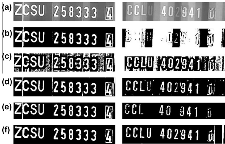
Fig. 16. Comparison of segmentation: (a) original images; (b) results of Otsu's method (Otsu, 1979); (c) results of Niblack's method (Niblack, 1986); (d) results of logical level technique (LLT) (Kamel & Zhao, 1993); (e) results of Sauvola's method (Sauvola & Pietikinen, 2000); and (f) our results.
