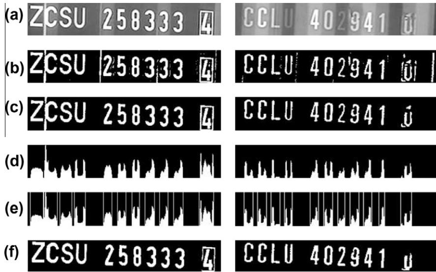
Fig. 15. Two segmentation examples: (a) original container-code images; (b) binary edge images; (c) denoised binary edge images; (d) vertically projected results; (e) different areas; and (f) final segmentation results.
