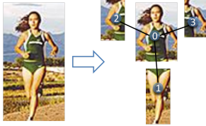
Figure 6. The four part star structured model. We divide the pose into four parts: legs, left-arm, right-arm, and upper-body.
