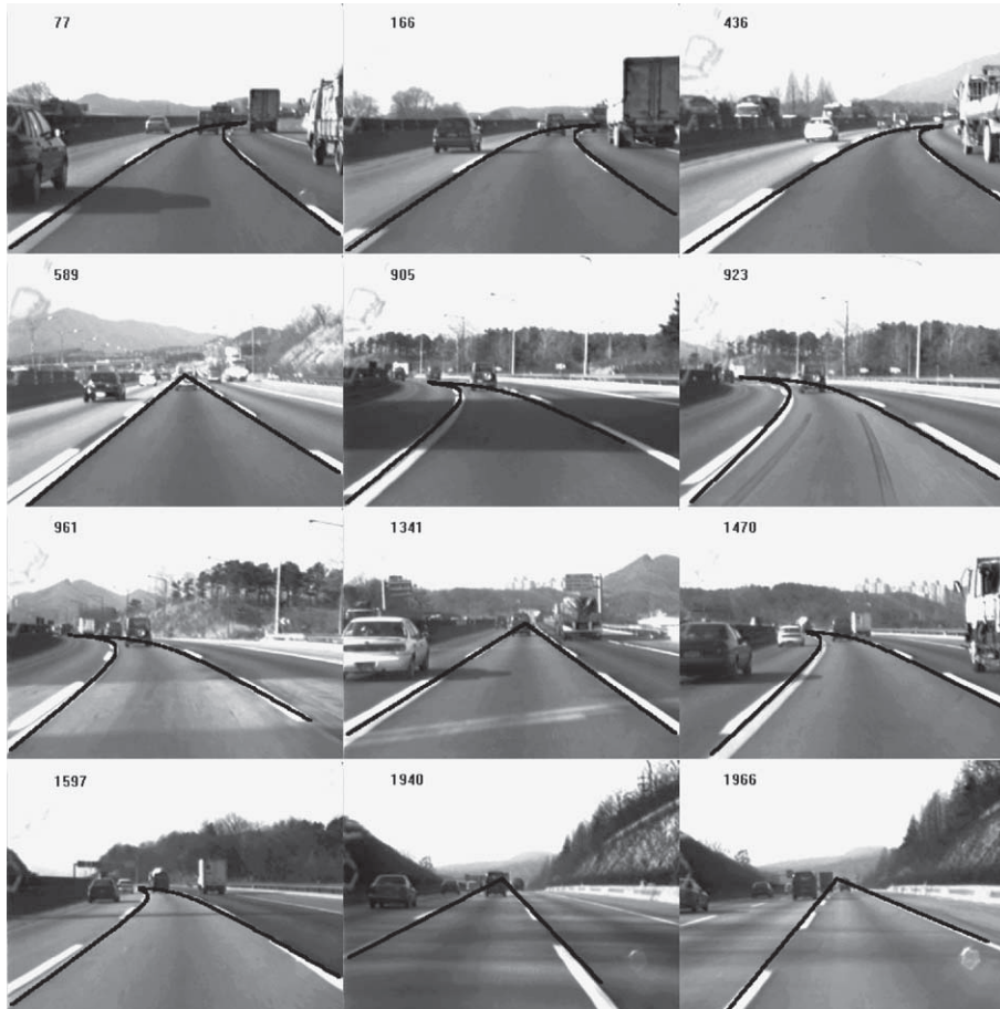
Fig. 9. The detected LCF in the road images. The solid lines indicate the detected LCFs. The result images were enumerated in the order of the capturing sequence of the road images.
