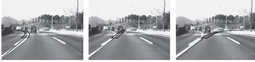
Fig. 4. The establishment of the LROI. The triangular pyramid shape is the LROI. Left: left-curved lane. Middle: straight lane. Right: right-curved lane.
